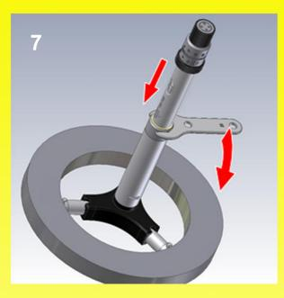
7 Afterward screw shaft tube with scale on extension and tighten well but moderately with special flat wrench.
