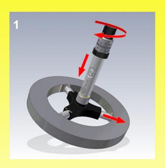
1 Insert the MICROTEST internal micrometer into the ring gauge or in triangle test gauge. screw out feelers until they are in contact with the side of the hole. Now turn ratchet half a revolution 5–6 times to obtain exact centring.
