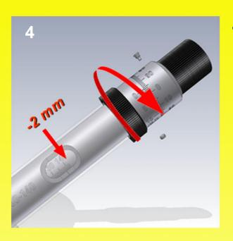
4 When Nonius screw is loosen and Allen screw is completely removed, screw knurled black ring underneath the Nonius counter-clock-wise exactly 2 mm, according to the mm-scale, upward.
