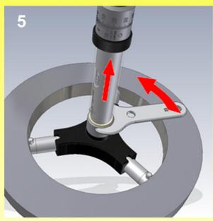
5 With the annexed special flat wrench loosen scaled shaft tube from housing and unscrew it counter-clock-wise by hand.
