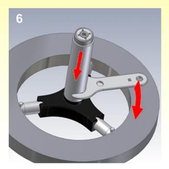
6 Screw the extension tube clockwise onto the housing and fix well but moderately with special flat wrench.
